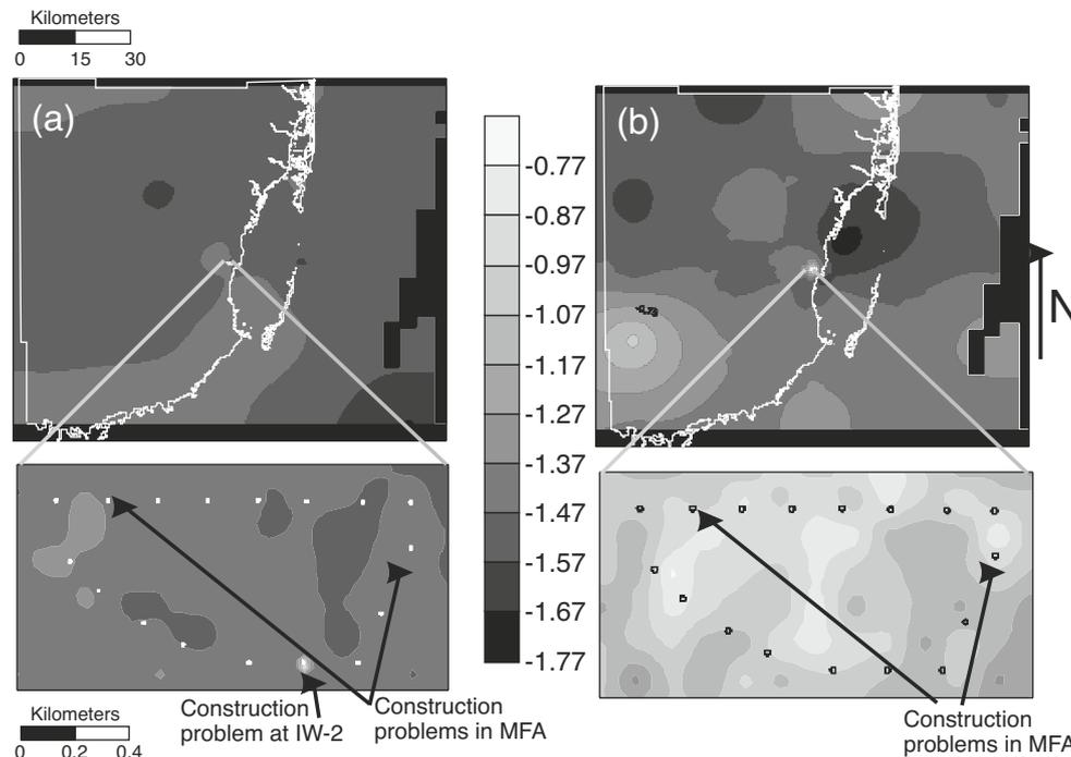
**Fig. 6** Calibrated log transformed vertical hydraulic conductivity fields (in m/day) for the Delray Dolomite (Fig. 3) for **a** calibration run 1 with construction problems for all three plumes, and **b** calibration run 3 which tests hypothesis 2 for the SE plume. Injection wells are the small white or black open circles
