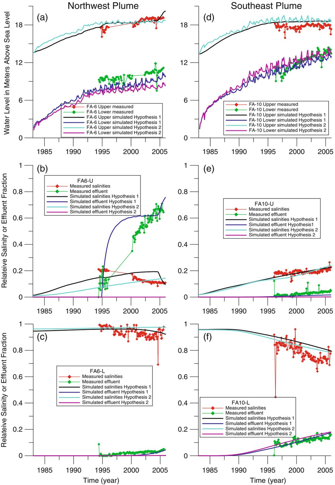
**Fig. 5** Calibration graphs for **a** water levels at FA-6, **b** relative salinity and effluent fractions for FA-6 upper, **c** relative salinity and effluent fractions for FA-6 lower, **d** water levels at FA-10, **e** relative salinity and effluent fractions for FA-10 upper, and **f** relative salinity and effluent fractions for FA-10 lower
