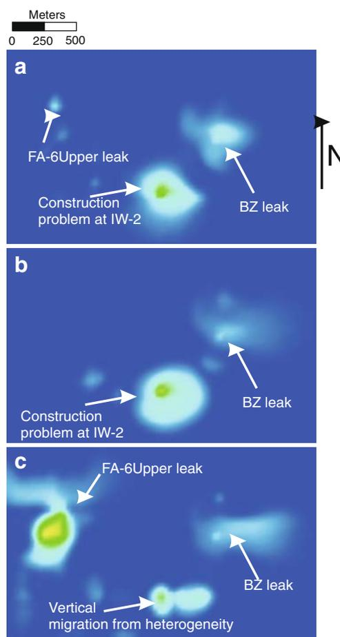
**Fig. 7** Map view of effluent in the MFA (Fig. 3) showing the migration of effluent from **a** calibration run 1 (which represents hypothesis 1 for all plumes), **b** calibration run 2 (which represents hypothesis 2 for the NW plume), and **c** calibration run 3 (which represents hypothesis 2 for the SE plume)
