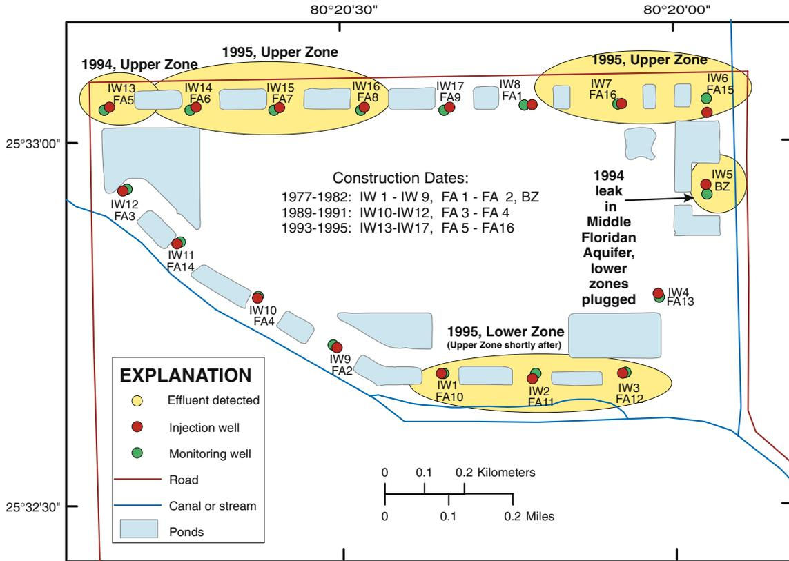
**Fig. 2** Map of wastewater treatment plant showing injection (*IW*) and monitoring (*FA* and *BZ*) wells. Areas where effluent has been detected in a monitoring well are shown in yellow
