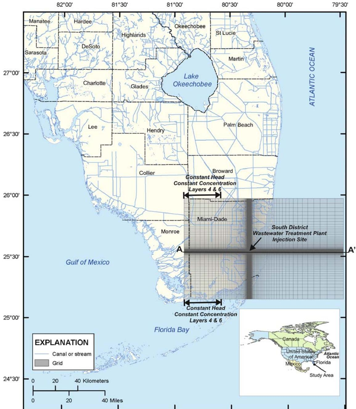
**Fig. 1** Map of Florida showing the site location, model grid, landward boundary conditions in model layers 4 and 6, and counties (shown as dashed lines)
