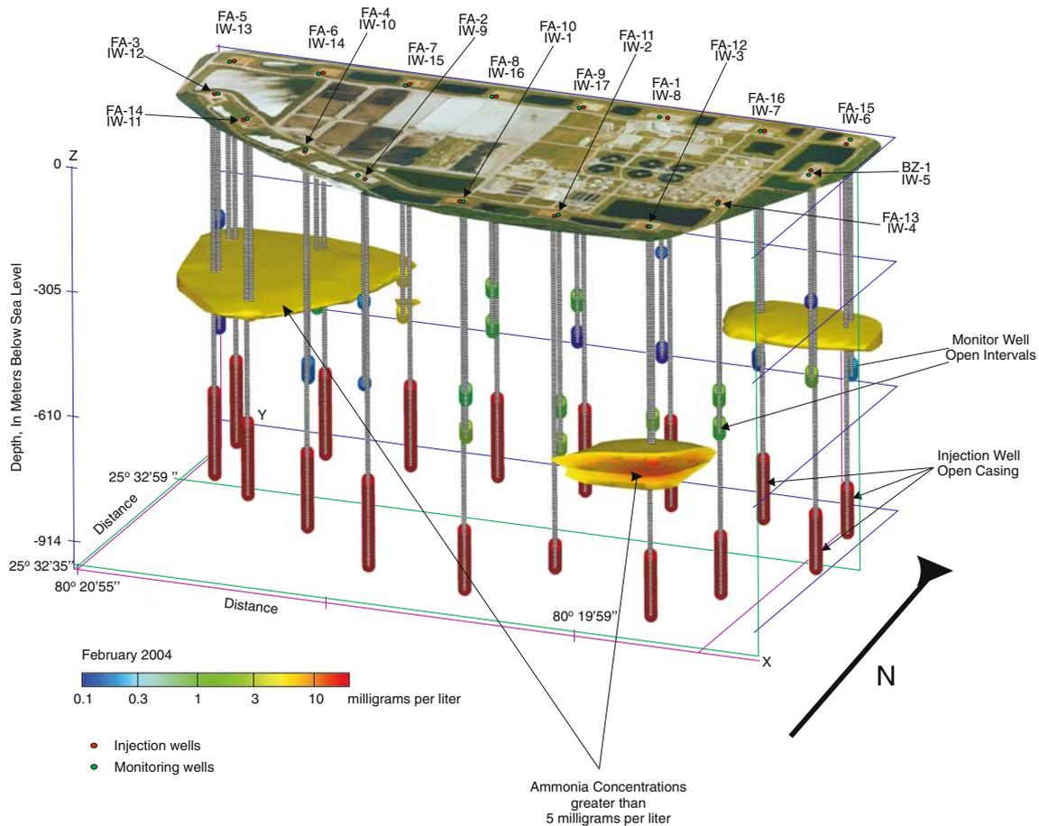
**Fig. 4** Three-dimensional visualization of the site showing the injection and monitoring wells. The three effluent plumes are represented as shaded areas where ammonia concentrations exceed 5 mg/L. The NE and NW plumes are in the MFA; the SE plume is in the MCU2
