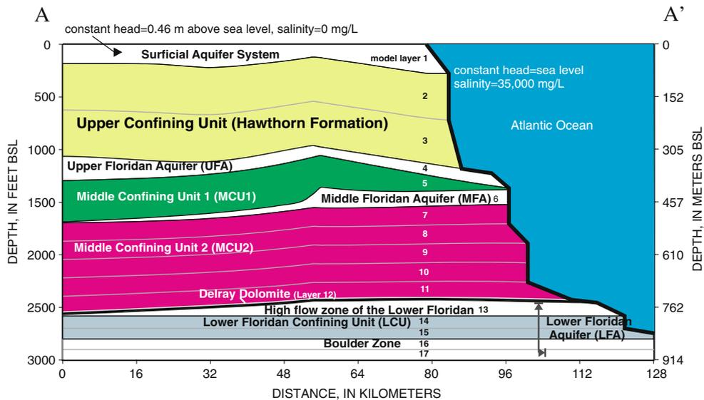
**Fig. 3** Cross section showing aquifer and confining units (Reese and Richardson 2008; McNeill 2002). Model layers 1–17 are also shown
